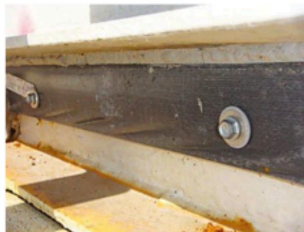
Eliminator isolator installed on existing double-bottom tank.
